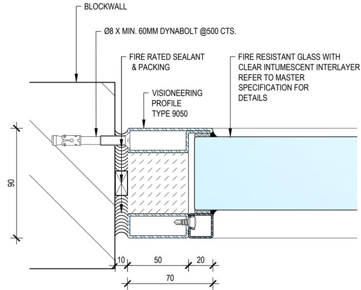
**1 JAMB DETAIL - CONCRETE FIXING**
